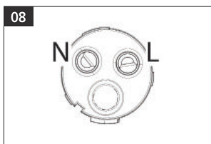
08 Connect the cables correctly to the core.
