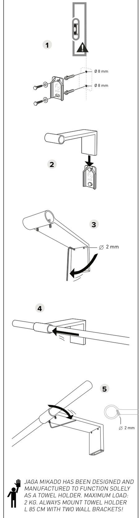
**JAGA MIKADO HAS BEEN DESIGNED AND MANUFACTURED TO FUNCTION SOLELY AS A TOWEL HOLDER. MAXIMUM LOAD: 2 KG. ALWAYS MOUNT TOWEL HOLDER L 85 CM WITH TWO WALL BRACKETS!**
