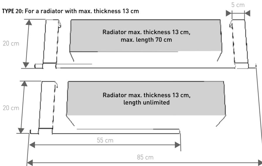
Always attach L85 using two brackets
