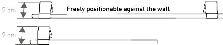
**TYPE 16:** For a radiator with max. thickness 9 cm
