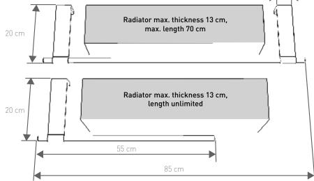
Always attach L85 using two brackets
