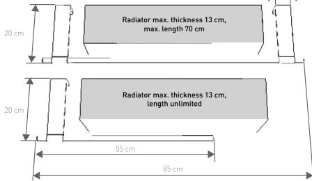
Always attach L85 using two brackets
