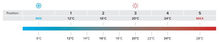
All TRV thermostatic heads are adjusted in a climatic chamber, free of external influences such as heat build-up, sunshine, etc. The number 3 corresponds to a temperature of approximately 20 °C (68 °F). The difference between each number is approximately 4 °C (7 °F), from bar to bar approx. 1 °C (2 °F).
