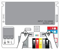
2. Press and hold down both the [-] and [+] button on the circuit board and switch on the power again. **The blue LED** will light up, followed by **the green LED** 2 seconds later and **the red LED** 4 seconds later. Release the buttons as soon as all 3 LEDs are flashing.
