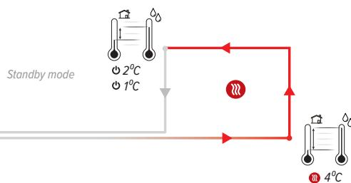
The device automatically enters the cooling mode as soon as the water temperature is 4°C lower than the room temperature. If the water temperature is less than 2°C lower than the room temperature, the device will automatically switch to standby.
