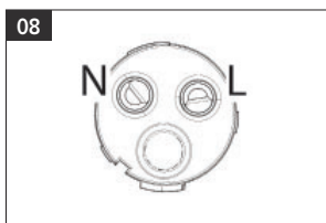
08 Connect the cables correctly to the core.
